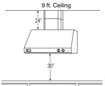
**9 ft. ceilings:** When the hood is installed 30" above the cooking surface, order two 12" duct cover accessories.
